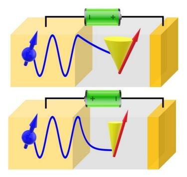
**Magnons on demand.** The new transistor starts with a spin current (blue) flowing up through a platinum plate and converts it to a flow of magnons (red). The rate of conversion can be controlled with a voltage, represented as a battery. A positive voltage (left) increases the magnon output, whereas a negative voltage (right) reduces it.
